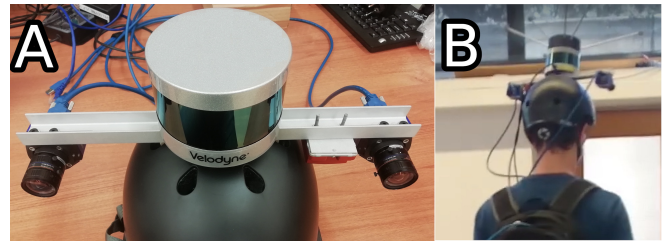
Fig. 9: The experimental setup with two MV BlueFox3-2016C-1112 cameras and Velodyne VLP-16 LiDAR without hardware trigger (A) that was used for indoor mapping when mounted on a helmet (B)
