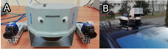
Fig. 10: The experimental setup with two MV BlueFox3-2016C-1112 cameras and SICK MRS6124 LiDAR without hardware trigger (A) that is used in automotive applications (B)
