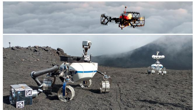
Fig. 1: Our Lightweight Rover Units (LRUs) [1] and drone ARDEA [2] test their skills for autonomous navigation, exploration, and sampling at a Moon-analogue site on Mt. Etna.
