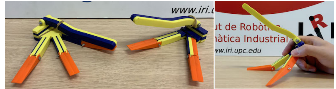
Fig. 3. Simple prototypes to evaluate the grasp geometries.
