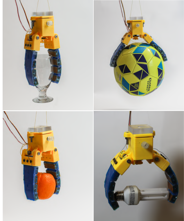
Fig. 1. An electrostatic/gecko-inspired adhesive soft gripper picks up and handles a wine glass, a soccer ball, an orange, and a lamp. The contributions of electrostatic/gecko-inspired adhesives are important to grasp steadily the wine glass, orange, and soccer ball.
