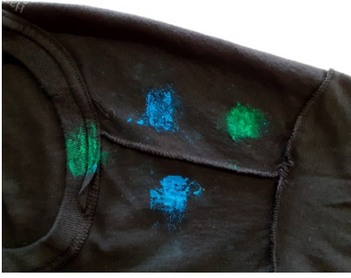
Fig. 6: Estimate of the fabric portion involved in the grasp, with and without the electromagnet exploitation (blue and green marks, respectively). A smaller portion produces less wrinkles, increasing the grasp precision.
