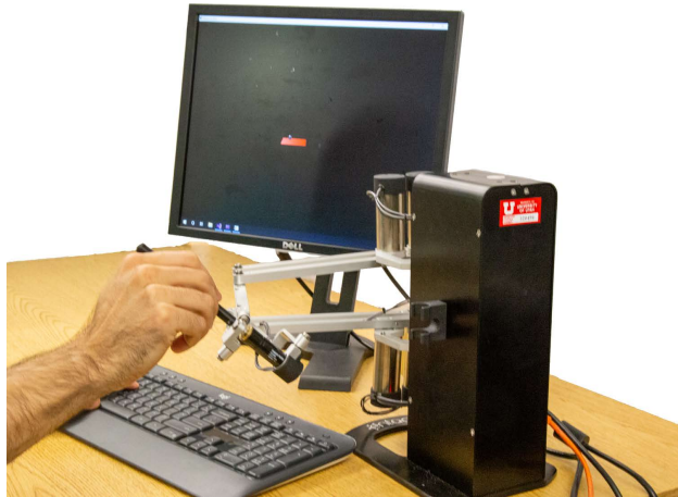
Fig. 2: The experimental setup. The subject holds the haptic device’s stylus, with his elbow resting on an armrest, and controls a proxy in a simple 3D virtual world. A dot was painted on the stylus, indicating where the subject should grasp it, with \|\mathbf{r}\| = 120 \text{ mm} . The user can use the keyboard to toggle between the surface properties and enter the final answer.
