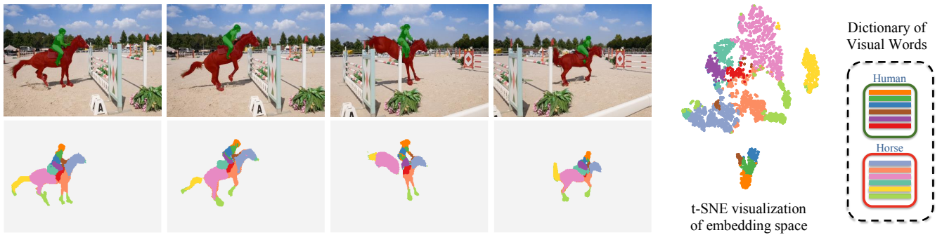
Fig. 1: Video object segmentation using a dictionary of deep visual words. Our proposed method represents an object as a set of cluster centroids in a learned embedding space, or “visual words”, which correspond to object parts in image space (bottom row). This representation allows more robust and efficient matching as shown by our results (top row). The visual words are learned in an unsupervised manner, using meta-learning to ensure the training and inference procedures are identical. The t-SNE plot [1] on the right shows how different object parts cluster in different regions of the embedding space, and thus how our representation captures the multi-modal distribution of pixels constituting an object.
