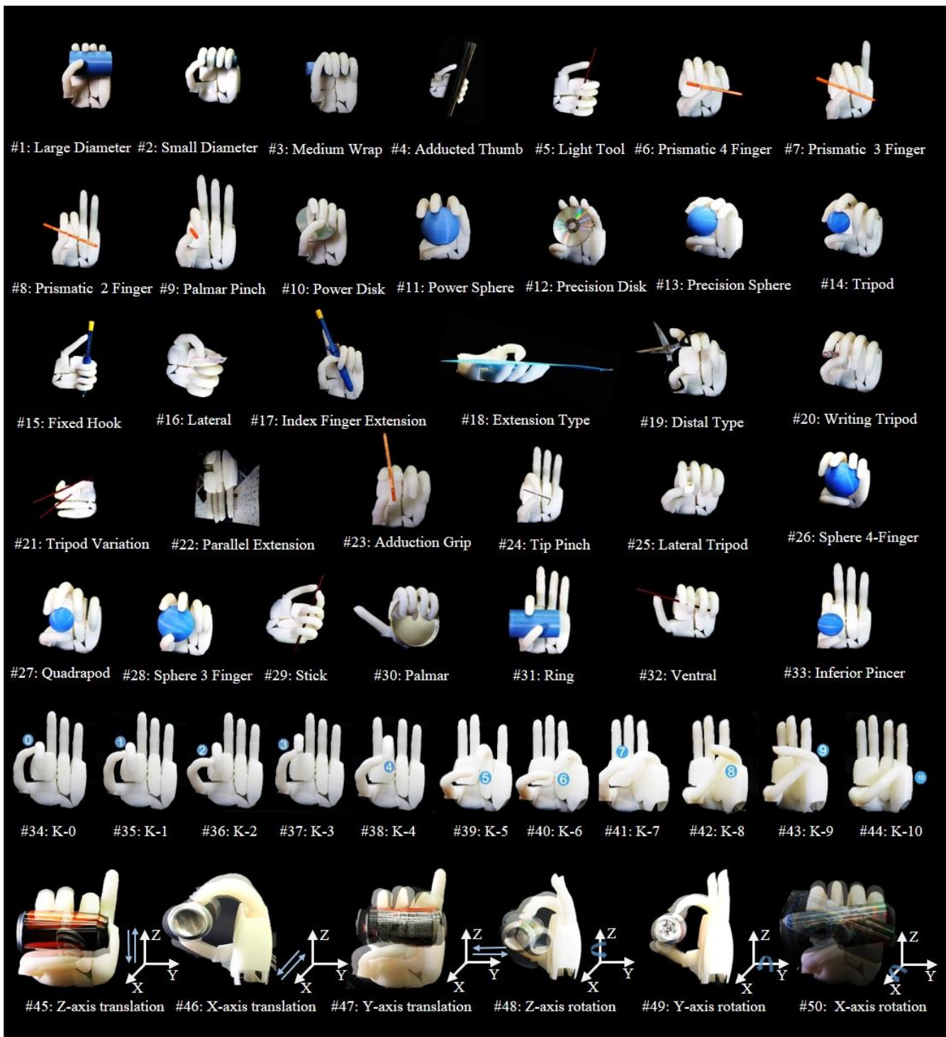
Figure 2. 50 hand dexterity benchmarks (HD-marks) achieved by S-22: (#1-33) present the realization of 33 grasping taxonomy tasks. (#34-44) present the achieving of 10 Kapandji tests. (#45) presents the Z-axis translation. (#46) presents the X-axis translation. (#47) presents the Y-axis translation. (#48) presents the Z-axis rotation. (#49) presents the Y-axis rotation. (#50) presents the X-axis rotation.
