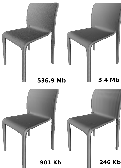
Fig. 1. Visualisation of 512^3 TSDFs. Non-compressed TSDF and various degrees of TT-compression
