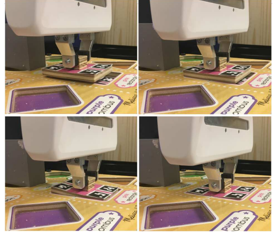
Fig. 6. Demonstration where the human operator moves the robot arm, via teleoperation, to complete the shape insertion task after model failure. We found that demonstrations worked best when the operator reset the shape to a position outside of the hole and performed a sliding motion into the hole.
