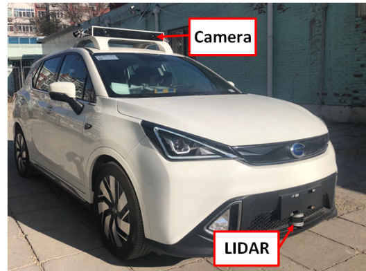
Fig. 5. Our self-driving car platform, equipped with monocular cameras and a LIDAR sensor.
