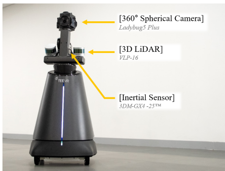
Fig. 8. Sensor system for data acquisition. Sensor measurements, acquired by a spherical camera, two 3D LiDARs, and an inertial sensor are employed to generate realistic 3D modeling [14].
