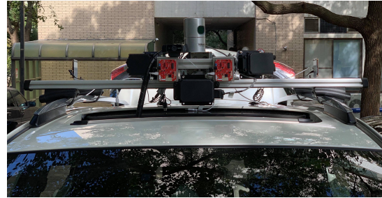
Fig. 1. Sensors on the test vehicle. One Velodyne HDL-32E LiDAR and three Delphi ESR radars are used in this work.
