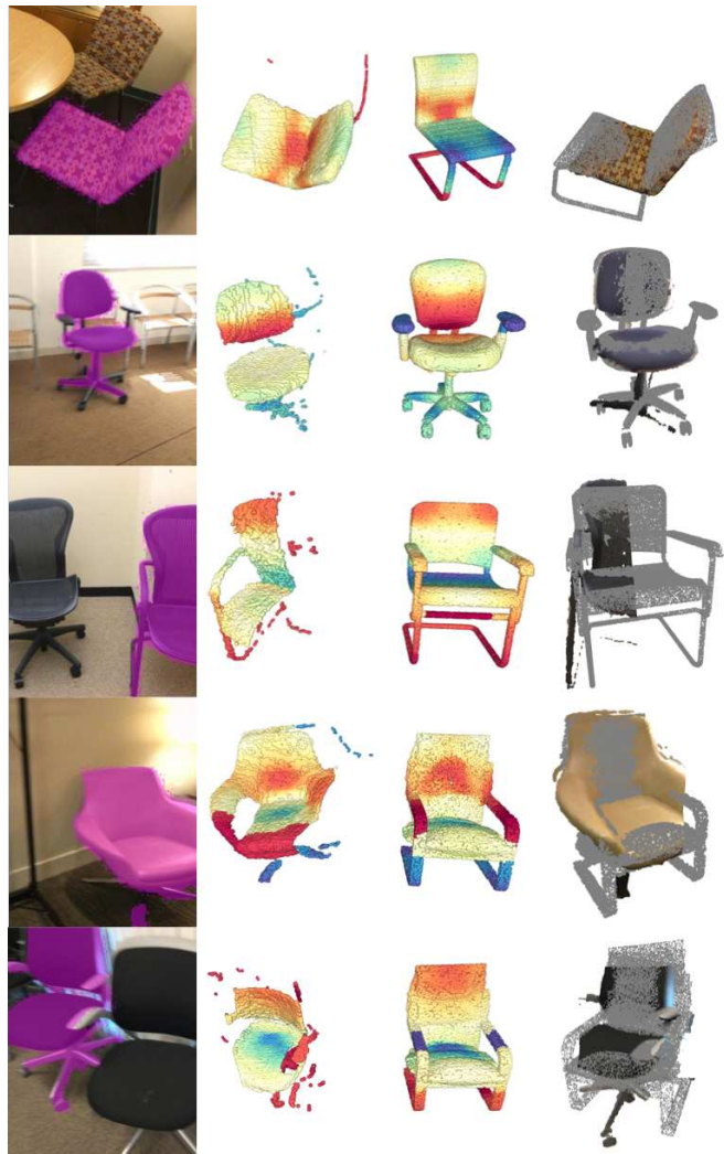
Fig. 8: Examples on matching the point cloud segmented from a single RGB-D image. Column 1: RGB images and object segmentation masks in purple. Column 2 & 3: color-coded point cloud features of the observed objects and the CAD models. Column 4: Alignment results with the CAD models painted in grey.
