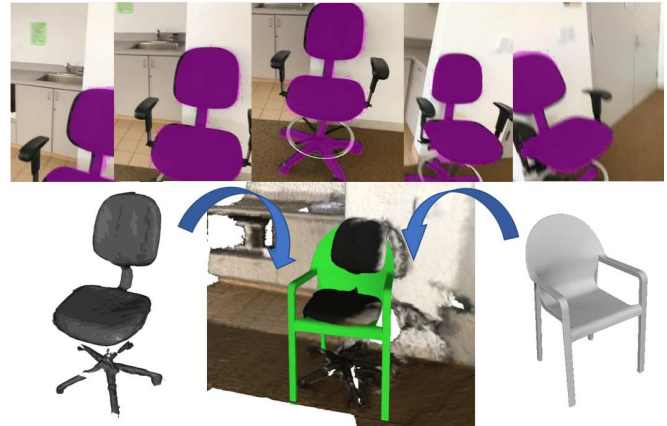
Fig. 1: A sequence of RGB-D images (top) may be used for object-level mapping. This paper focuses on the important subproblem of category-level registration. A partial object point cloud (bottom, left) may be generated from object detection, segmentation, and tracking (top, purple). A not-identical CAD model (bottom, right) needs to be aligned to the observed point cloud (bottom, middle) in order to generate an object-level map.
