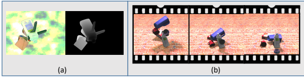
Fig. 4. Comparison of Domain Randomization (DR) against Physically Plausible Domain Randomization (PPDR). (a) DR directly renders using a sampled object pose. Notice the penetration between objects, which can introduce undesired bias to depth data. (b) In PPDR, a randomly sampled pose serves as initialization for physics simulation. Rendering is performed over the stable object pose. The domain invariant, penetration-free property can then help to effectively align the synthetic and real domains.
