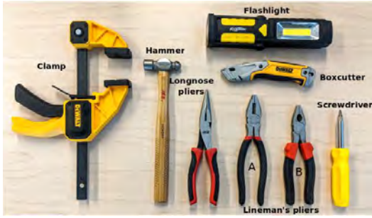
Fig. 4: Objects in our custom dataset. The clamp has one prismatic joint. The three sets of pliers each have one revolute joint. The other four objects are treated as rigid. The objects are separated into parts based on the presence of both affordances and articulations.
