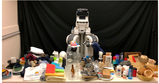
Fig. 1. The PR2 used a spectrometer and near-field camera to estimate the material of 144 everyday objects.
