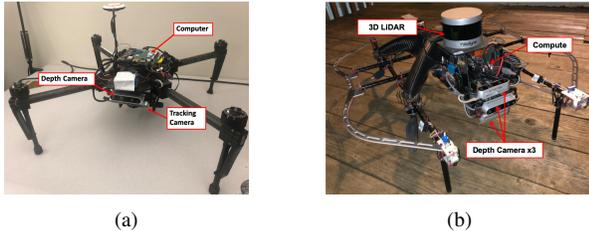
Fig. 11: (a) shows the DJI M100 used in the outdoor forest environment and (b) shows the custom quadrotor used in urban subterranean environments.
