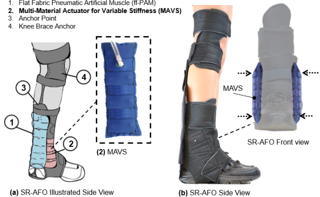
Fig. 1. Design of the SR-AFO exosuit with an anchoring strap on the knee (4) and a connecting strap (3) to the inflatable fabric-based actuator for plantar/dorsiflexion support (1). The SR-AFO is shown incorporating the Multi-material Actuator for Variable Stiffness (MAVS) in (2).
