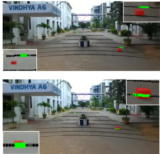
Fig. 6: (a) Point Cloud projection using calibration matrix obtained through [21]. (b) Improved calibration using our method. We can observe how projection error becomes more significant for farther obstacles.
