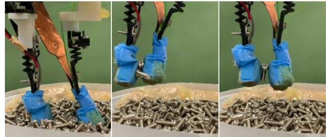
1. Grasp multiple screws 2. Perform manipulation 3. Obtain a single screw
