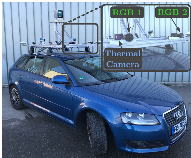
Fig. 3. Our stereo RGB and thermal camera rig mounted on our data collection vehicle.
