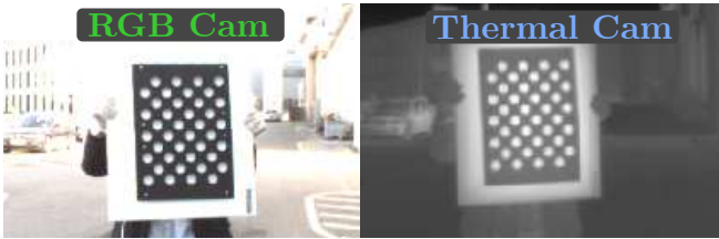
Fig. 4. Our calibration board placed in front of a heating panel is visible in the RGB and thermal domain. We record multiple image-pairs covering the whole camera frustum and obtain the calibration parameters with Kalibr [8]. This method is used as a baseline for our target-less calibration approach.
