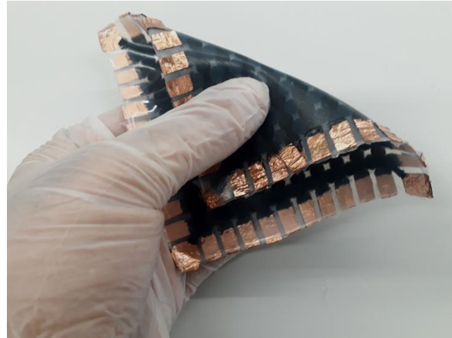
Figure 1: SCEEP, a silicon-based capacitive skin, is highly stretchable and foldable.
