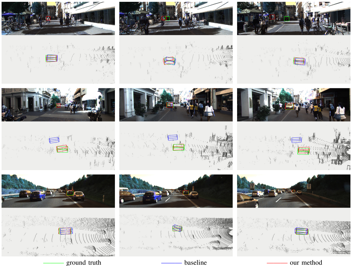
Fig. 4: Comparisons of our approach with the state-of-the-art tracker when setting the 3D template frame as the previous predicted result. Experiments show that our method is more robust due to introducing RGB information, and our method can achieve stable tracking even with the very sparse long-range point clouds. Besides, in the occasional case when 2D module passes inaccurate results, our method remains significantly accurate in tracking.
