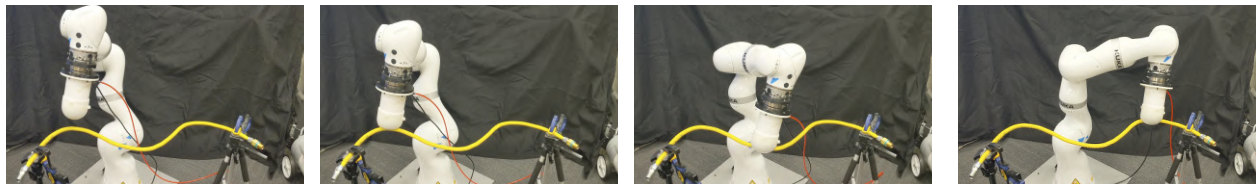
(a) Robot begins its policy rollout above the obstacle. (b) Robot lowers itself onto the pipe and follows the edge. (c) Contact is maintained during a dip in the -z direction. (d) Robot continues to contact the pipe along a lateral bend.
