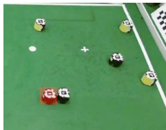
Fig. 6: Take-the-Treasure running on SSL RoboCup robots. Yellow robots are opponents. Highlighted robot currently has the treasure.
