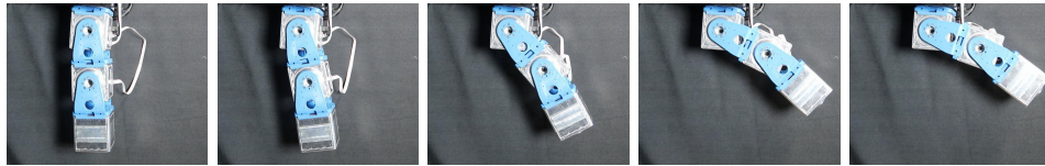
Fig. 4. Photo-sequence of the the last iteration of the slow minimum jerk trajectory in the heavy payload scenario.
