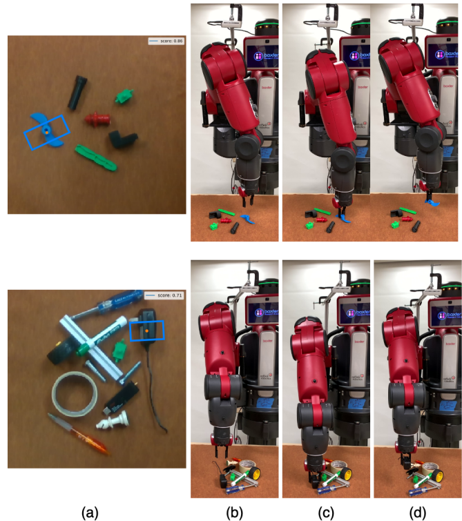
Fig. 5: Example of robot grasping adversarial (top) and household (bottom) objects. See attached video for complete run. (a) Grasp pose generated by inference module. (b) Robot approaching the grasp pose. (c) Robot grasping the object. (d) Robot retracting after successful grasp.
