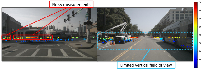
Fig. 2: Limitations of Radar measurements. (Left) Noisy measurements and (Right) Limited vertical field of view.
