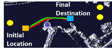
Fig. 7: The simulated robot model moves around a static obstacle to avoid colliding with it.
