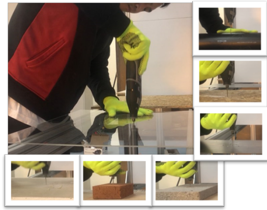
Fig. 3: Selected tool performance test: acrylic sheet, PVC pipe, plywood board, metal sheet, concrete, brick, and drywall (clockwise, inset)
