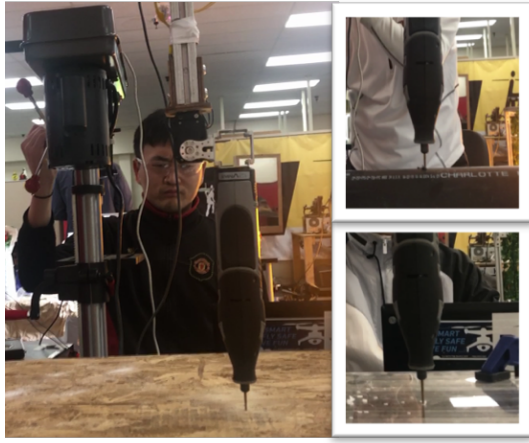
Fig. 7: Haptic drill press on plywood board (left), PVC pipe (Top inset), Acrylic sheet (Bottom inset)
