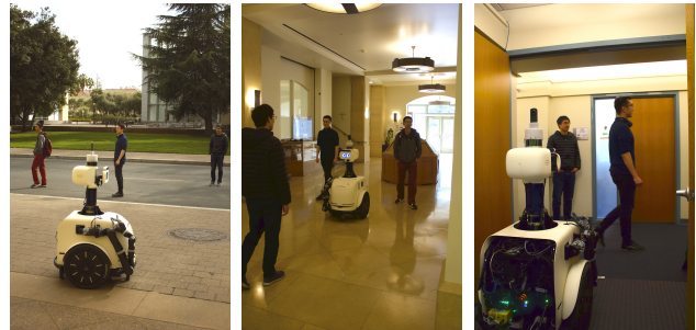
Fig. 5: We conduct on robot experiments in 3 different scenes, shown above, with a varying number (1 - 7) of people, at different distances (1 - 10m), with different types of human trajectories (moving and stationary), and with JackRabbit both moving and stationary. We aimed to conduct experiments in diverse, real-world conditions. The above images depict our experimental setup.
