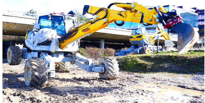
Fig. 1. Top : A walking excavator has five limbs; an arm, and four legs with a wheel at the end of each leg. They usually operate in muddy and slippery conditions, which requires motion plans with large stability margin. Bottom : HEAP balancing on three legs while performing a stepping maneuver. A video demonstrating all the motions accompanies this submission.
