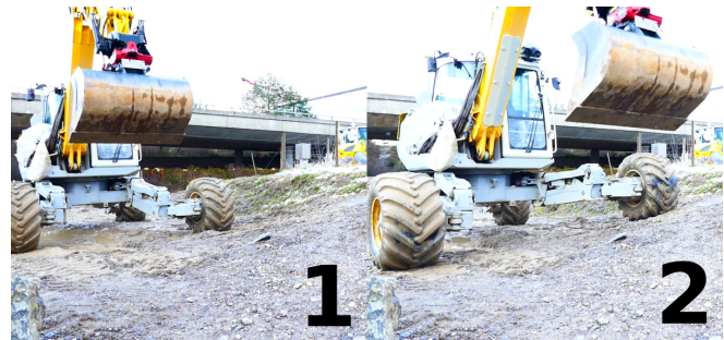
Fig. 7. Left to Right : HEAP driving forward over a small hill. The front leg adapts its height to the ground height, despite motion planner producing plans under the flat ground assumption.
