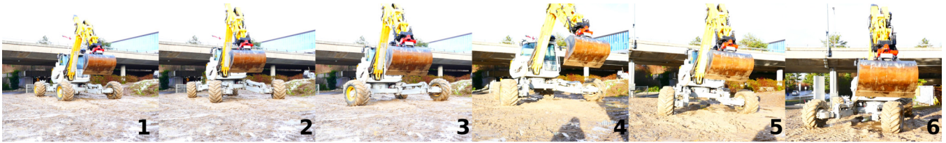
Fig. 9. Left to Right: HEAP performs a driving maneuver. The base is commanded to move forward and left (frames 1-3). Subsequently, we command the machine to drive back to the starting point (frames 4-6). The planning and control pipeline naturally discovers the crab steering mode of the machine.
