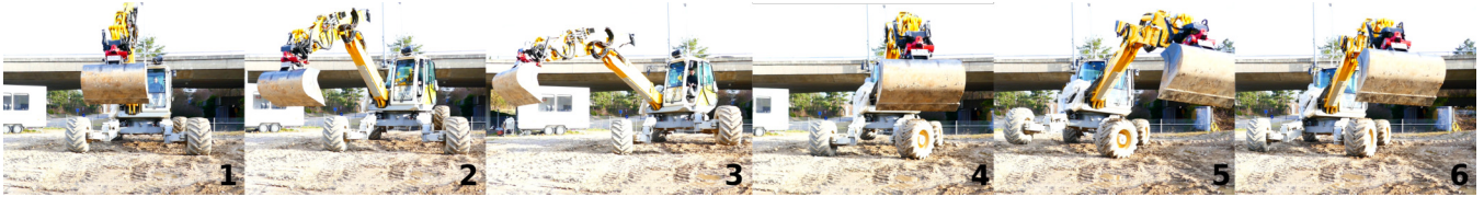
Fig. 10. Left to Right: HEAP performs a stepping maneuver and reorients its base by 30^\circ . The gait pattern requires it to lift the legs in the following order { LH, LF, RH, RF }. The machine cannot complete the maneuver without using the arm for balancing (e.g., in snapshot 3).
