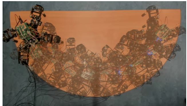
Fig. 11: Overlay of all the locations selected to place foot as the robot moves anti-clockwise around a semi-circular table. The robot correctly sensed the edge along the entire semi-circular section of the table.
