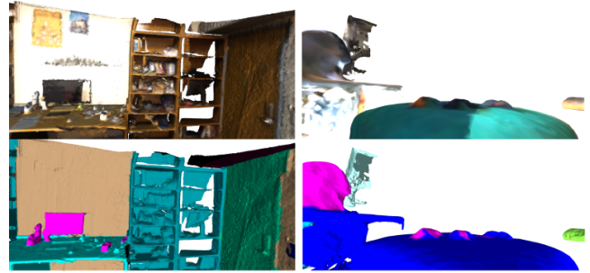
Fig. 3: Examples from ScanNet showing annotation inaccuracy. Small objects are incorrectly labeled, either under-segmented or not separated from the supporting structure. Top: original scan. Bottom: annotation with objects in pink.
