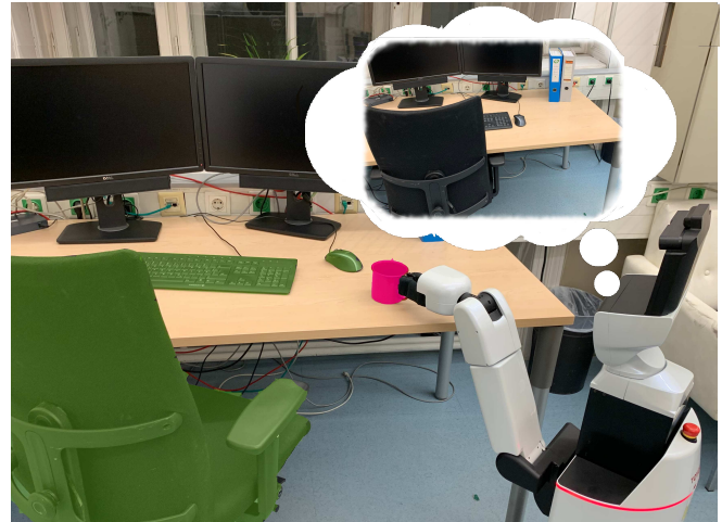
Fig. 1: A household robot tidying-up a room. It compares a previously acquired reference map to the current state of the environment. Although the chair and other permanent objects moved slightly (colored in green), only the mug (colored in pink) should be detected as novel and therefore tidied-up.
