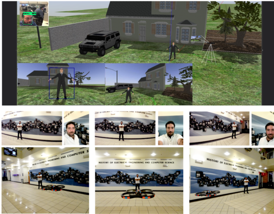
Fig. 7. Evaluating SelfieDroneStick in a custom simulation environment and in real-world using the Parrot ARDrone 2.0.
