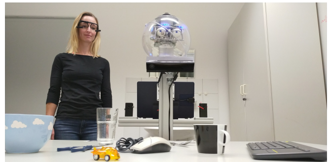
Fig. 1: Without specialized pre-training, the robot does not know the objects in front of it. Nonetheless, through our proposed approach, the robot is capable of detecting these unknown objects based on gaze-based human-robot interaction without any training instances.
