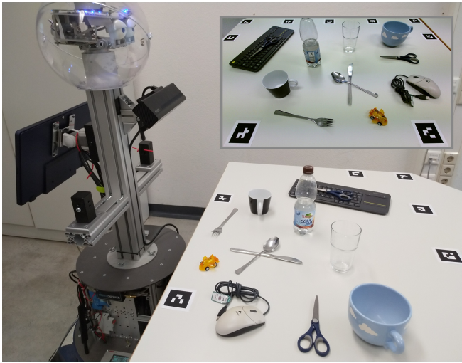
Fig. 3: With a Microsoft Kinect v2 the robot sees different objects on a table: Keyboard, scissors, cups, bottle, fork, knife, spoon, mouse and a small toy car.
