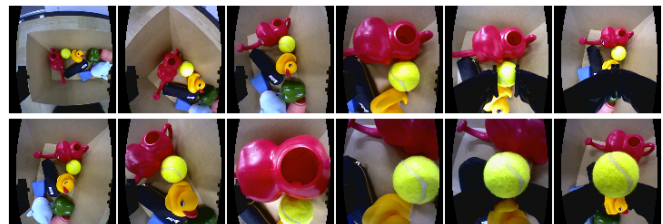
Fig. 8. A sequence of wrist camera observations from a successful attempt to grasp the tennis ball.
