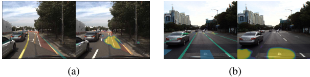
Fig. 10. Failure cases where partially visible objects are falsely detected as changes. (a) Only part of the lanes are visible on a partially paved road. (b) Arrow truncated at the edge of the image frame.
