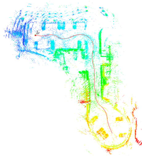
Fig. 7. A 3D map from accumulated radar scans with estimated calibration parameters. The outlines of parked cars can be clearly seen.
