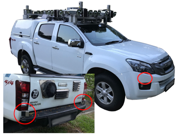
Fig. 1. The vehicle platform. Four 3D LiDAR sensors are mounted on the roof rack. Red circles mark the locations of a radar located behind the front bumper and two radars mounted on the rear bumper.
