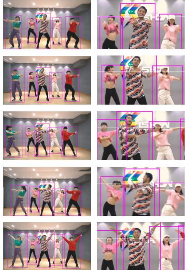
Figure 7. The result of MOV in tracking several dancers. The interval of the image series is 1 second. The left column is the video scene and the detection results by YOLOv3 and the right column is the camera screen. We only track the three persons in the middle.
