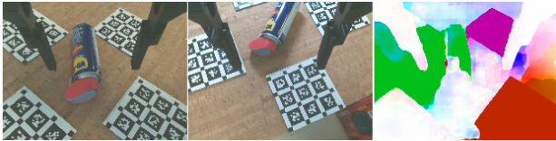
Fig. 6. Example of erroneous optical flow resulting from a large rotation and limited overlap between the two images. Examples of good flow are shown in Fig. 1 and Fig. 2. White indicates zero flow magnitude.
