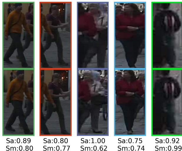
Fig. 1: Illustration of detection association using our proposed model. From top to bottom, bounding box detections at frame t - 1 and correctly associated bounding box detections at frame t . The corresponding appearance S_a and motion affinity S_m values ranges between 0 – 1 (0 represent lowest similarity and 1 highest similarity).
