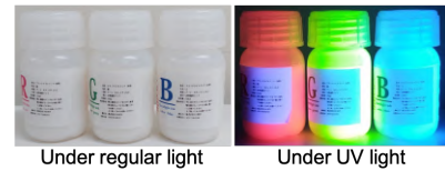
Fig. 2: Fluorescent paint under regular light and UV light
