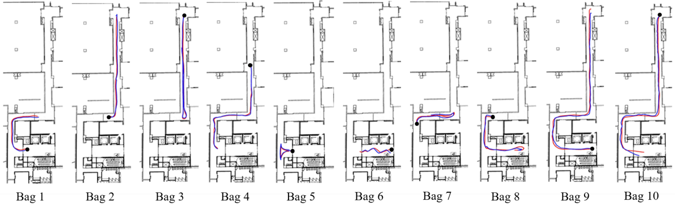
Fig. 5. State trajectories of AMCL and SGD on a floor plan as input map. State trajectory produced by both SGD state tracker and AMCL are still relatively consistent despite minor perspective distortion.
