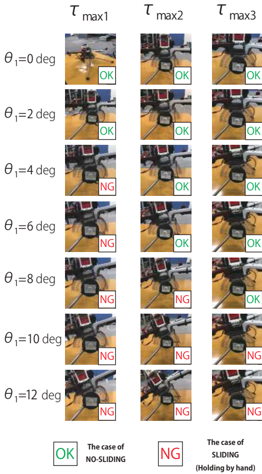
Fig. 13. Experimental verification of the frictional torque of the passive joint
