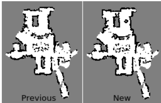
Fig. 13. Disconnected occupancy map. Underlying cause for disconnected wall in Fig 12
