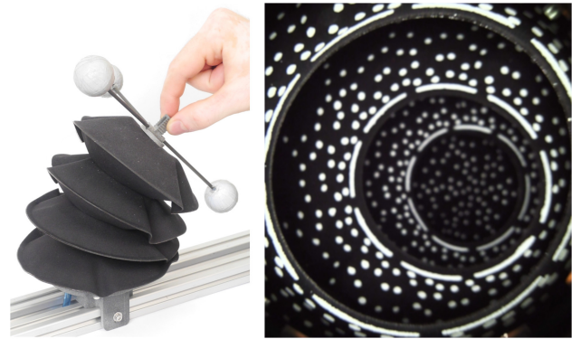
Fig. 1. Left: Manually deflected inflatable linear soft actuator with integrated camera. Markers for an external motion capture system are mounted on top for the acquisition of ground truth data. Right: Image from the integrated camera showing the employed pattern. The proposed sensing method is used to predict the tip position located on the grip, using only images from the integrated camera.
