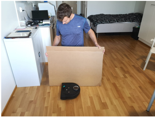
Fig. 4: A human (Markku) with cardboard, acting as a VWG, haptic renderer and display for a Neato vacuum cleaner robot.
