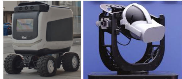
(a) (b) Fig. 1: (a) A Kiwibot food delivery robot. (b) A robot in full VR: An Optofidelity Buddy 3 wearing an Oculus Go headset.
