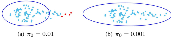
Fig. 6. The Gaussian 1-sigma ellipse with a different choice of \pi_0 . The man is waving his hand and the shape of point cloud has a great change over scans. When using a larger \pi_0 , points away from the Gaussian center are snatched by the clutter model.
