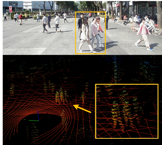
Fig. 1. Hybrid view of a crowd scenario. The point cloud is collected by four RS-LiDAR-16 scanners on our intelligent delivery robot. People marked by the yellow box are in close proximity and it is challenging to cluster each individual using spatial segmentation methods.
